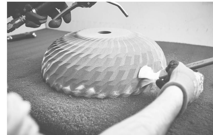
Loose sand is removed from the product after the 3D printing.
